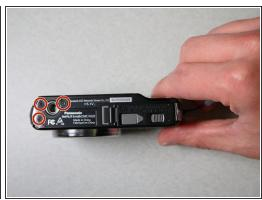
Remove all screws (Phillips #000 head) from the sides and bottom of the camera.
