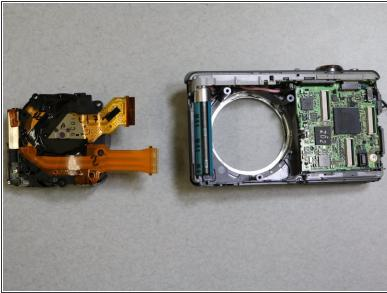
Remove the lens from the camera carefully. You can do this simply by grabbing it with your fingers and pulling out gently.
