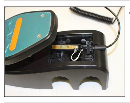
If this small sensor is broken, it is time to buy a new foot pedal and replace the broken one.
