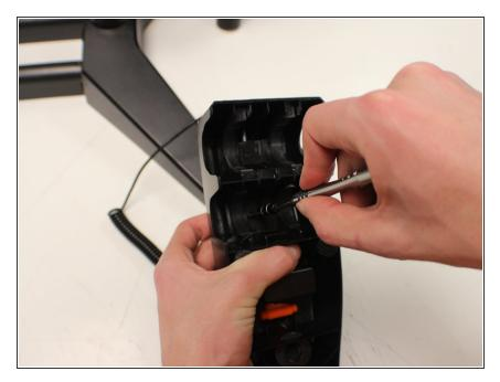
Remove the two Phillips size J0 screws holding the cover plate on the top of the foot pedal.
