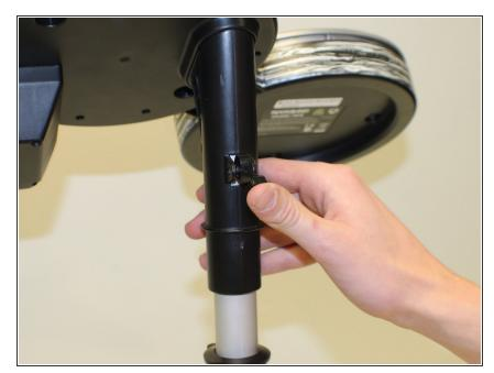
• Flip the leg retention clips on the back of the upper assembly down.
