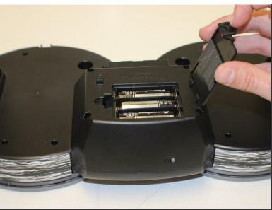
Remove battery door from the bottom of the drum set
