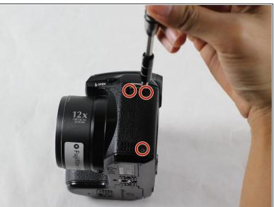
Use the Phillips PH00 screwdriver to remove all the 0.5mm screws on the side.
