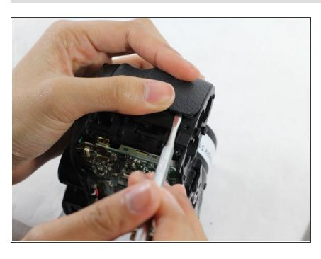
Using the metal spudger, place it in between the leather grip and the black plastic compartment
