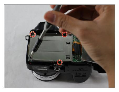
Use the PH00 screwdriver to unscrew the 0.5mm screws located near the top left corner, top right corner, and bottom right corner.
