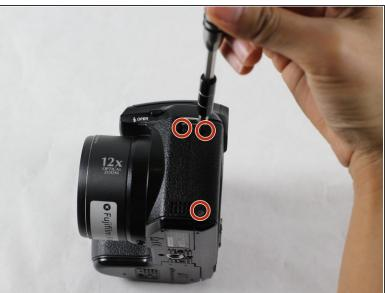
Use the Phillips PH00 screwdriver to remove all the 0.5mm screws on the side.
