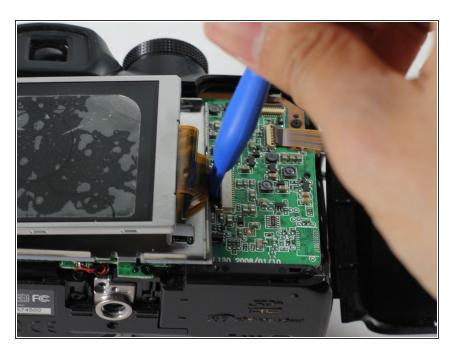
Once the screen is out, you will realize that it is still connected to the ribbon cable. To unplug this ribbon cable, use a plastic opening tool to pull up and to the left on the ribbon cable connector and release the ribbon cable.
