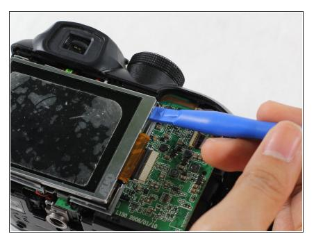
Use a plastic opening tool to lift up the right side of the display screen.
