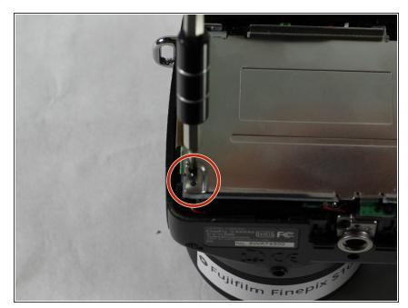
Using your PH00 screwdriver, unscrew the 0.5mm screw located on the bottom left hand corner where the display screen used to be.
