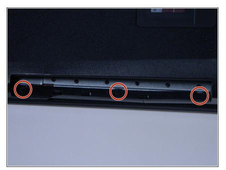
Remove the three screws located where the DVD ROM once was, on the screen side of the laptop.
