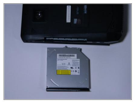
Remove the DVD ROM on the side of the computer, by pulling it out. If necessary, use a plastic opening tool.
