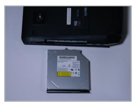
Remove the DVD ROM on the side of the computer, by pulling it out. If necessary, use a plastic opening tool.
