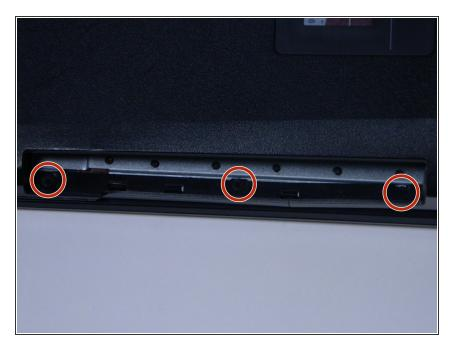
Remove the three screws located where the DVD ROM once was, on the screen side of the laptop.
