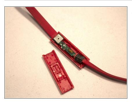
Remove this piece to expose the inner workings of the microphone.
