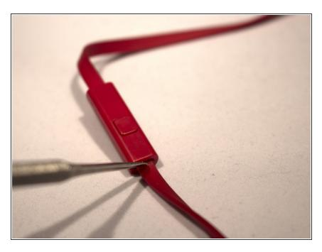
Using the metal spudger as a prying tool, gently remove the plastic casing around the microphone.
