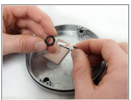
Remove the 1/2" hex nut holding the cable in place to the metal base with a 1/2" open-ended wrench.
