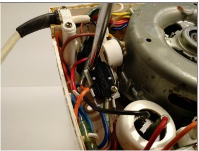
Remove the two 19 mm Phillips #2 screws holding the safety switch in the bracket.
