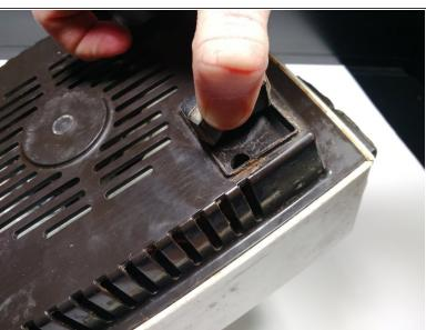
Remove the four 18 mm Phillips #2 screws from the bottom by prying up the rubber feet to access the screw hole.
