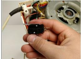
• Pull off the three wires on the safety switch with your hand by firmly grabbing the wires at the base.
