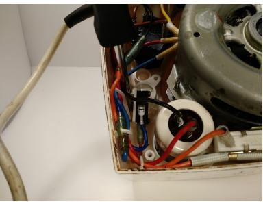
Remove the two 14 mm Phillips #2 screws holding in the safety switch bracket.
