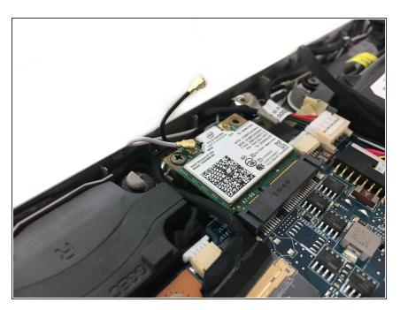
Locate the Wi-Fi/Bluetooth card, and remove the two wires connected to the card with your hands.
