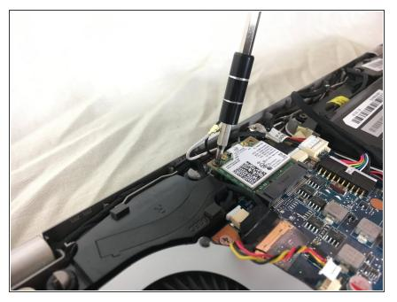
Unscrew the single 2.5x6mm holding down the card onto the board with your Philips #0 screwdriver.
