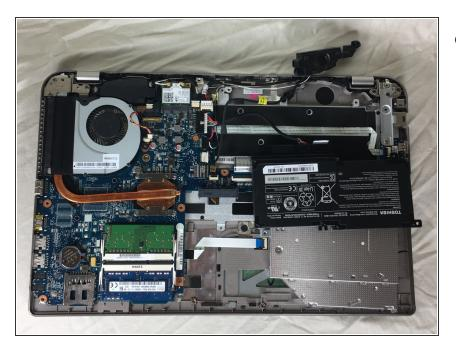
Remove the battery from the laptop after it has been completely disconnected.
