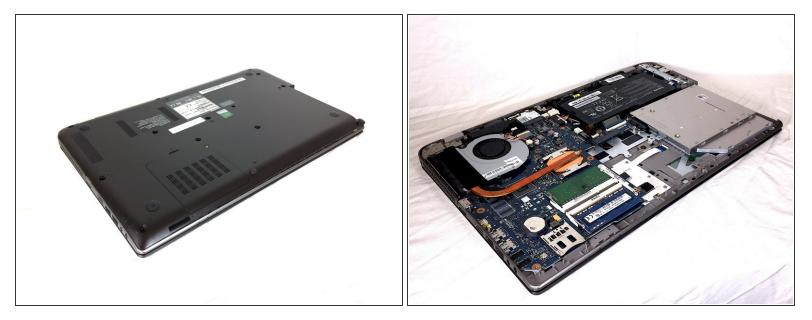
Remove the bottom cover of your laptop. For instructions on how to do this, take a look at the <u>Toshiba Satellite P55-A5312 Back Cover Removal Guide</u>
