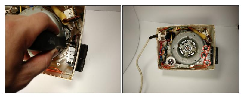
• Remove the three 12 mm Phillips #2 screws from the power switch assembly.
