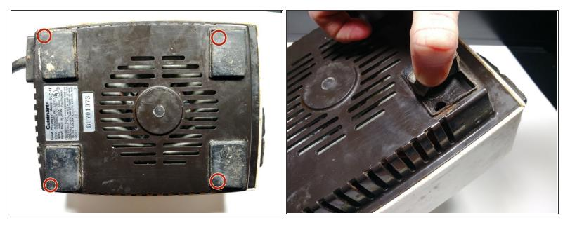
Remove the four 18 mm Phillips #2 screws from the bottom by prying up the rubber feet to access the screw hole.
