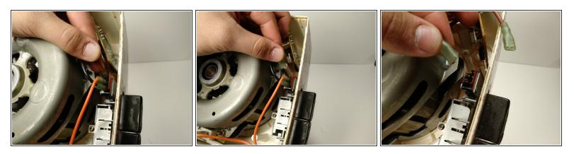
• Pull out the three wires coming out of the power switch assembly by firmly grabbing the base of the wires and pulling.
