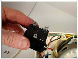
• Pull off the three wires by grabbing from the base of the wire.
