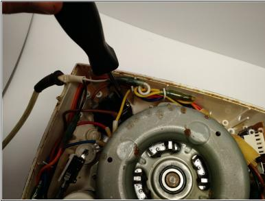
• Remove the two 15 mm Phillips #2 screws on the automatic circuit breaker.
