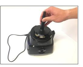
Using a #2 Phillips head screwdriver, remove the four 10 mm screws and pull the shaft straight upwards to uncover gears.
