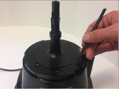
Use the nylon spudger to remove the plastic screw covers.
