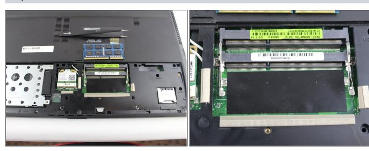
Now simply remove the ram by pulling it out using a set of pliers to be safe and careful not to damage the ram.
