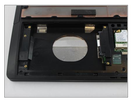
Remove the hard-drive. It will be connected to the integrated sata-port in the device.
