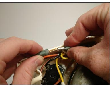
Pull apart the two wires of the power cable at their connections as shown.
