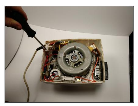
Remove the two 62 mm Phillips #2 screws from the cable retaining clip.
