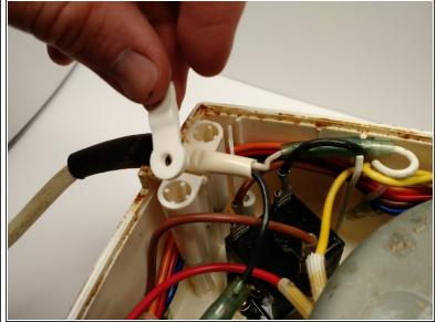
Lift off the cable retaining
