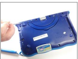
Remove all screw caps from the back panel using a metal spudger.
