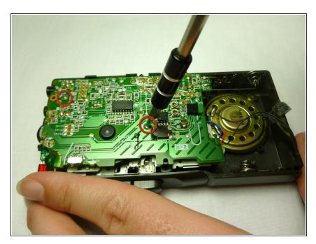
Using a #00 Phillips screwdriver, remove the two 1.4x3 mm screws securing the motherboard.
