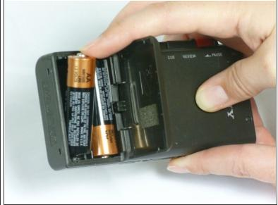
Lift the cover and remove the batteries.
