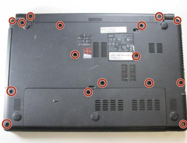
Remove the 16 2.5 x 8mm Phillips #0 screws from the back panel.
