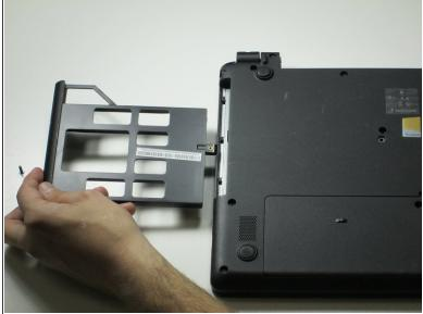
Slide out the plastic insert located on the left side, and remove, before returning the laptop to the face-up position.
