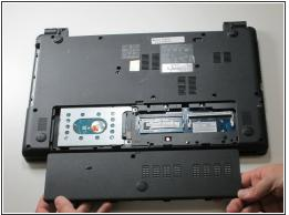
• Remove the back panel by carefully disengaging it around the edges and then pull upwards.
