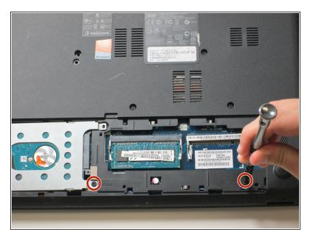
Unscrew the two remaining 2.5 x 8mm Phillips #0 screws from inside the bottom panel as designated in the image.
