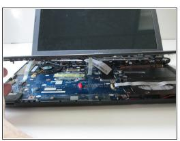
(i) Carefully detach the top panel of the laptop and slowly lift it up to reveal the internal components.
