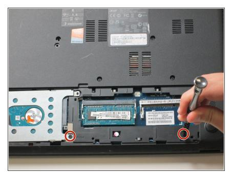
Unscrew the two remaining 2.5 x 8mm Phillips #0 screws from inside the bottom panel as designated in the image.
