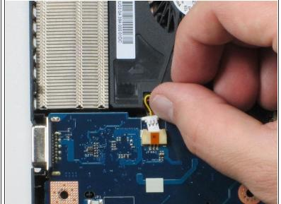
Remove the electrical wiring from its connecting port.
