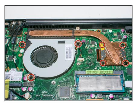
Remove the seven 4mm Phillips #0 screws holding the heat sink/fan assembly onto the motherboard.
