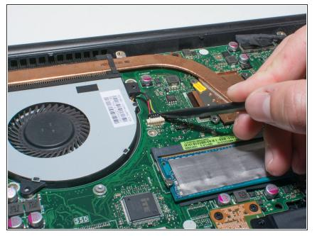
Using the spudger, unplug the fan from the motherboard connection by carefully pushing on both sides of the connector.
