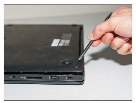
• Use the spudger to pry open the rear cover at either hinge.
