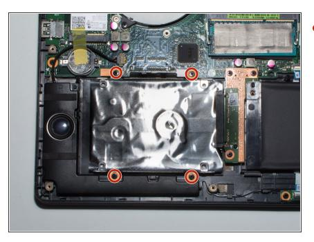
Remove the four 3mm Phillips #0 screws shown.
