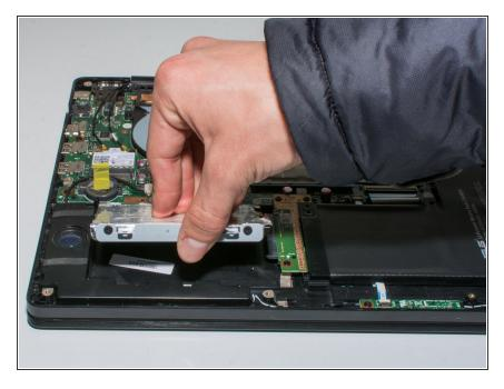
Once the hard drive has been removed from the connector, use your thumb to get under and lift the hard drive out.
