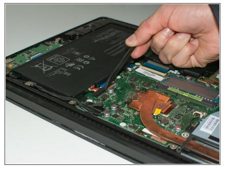
• Using the spudger, carefully remove the power cable connecting the battery to the rest of the laptop.
