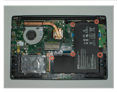
Remove the five silver 4mm Phillips #0 screws holding the battery to the laptop.
