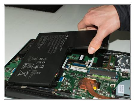
• Once the screws and cable are removed, carefully lift the battery from the laptop.
