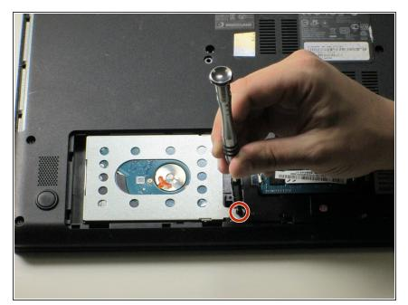
Remove the other 8mm Phillips #0 screw holding the hard drive to the rest of the laptop.
