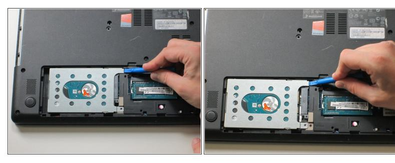
Slide the hard drive to the left using a plastic opening tool.
