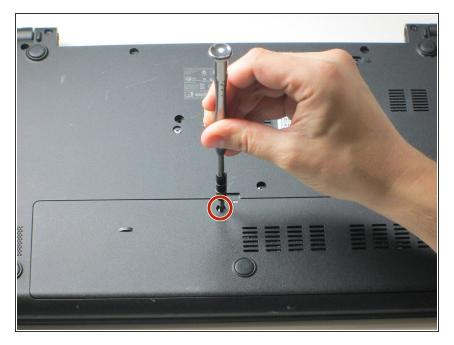
Unscrew the one 8mm Phillips #0 screw from the bottom panel.
