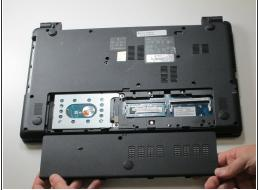
Remove the back panel by carefully disengaging it around the edges and then pulling upwards.
