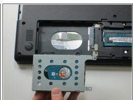
To remove the hard drive, pull up and to the left using the plastic tab as shown on the left side of the hard drive.
