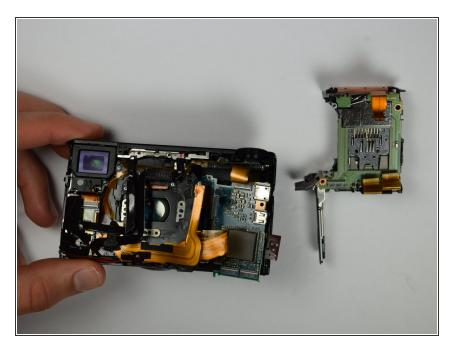
Remove the SD card holder. It should easily come out because all of the prerequisite screws were already removed.
