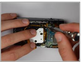
Using Philips Screwdriver, remove the four screws as marked on the picture
