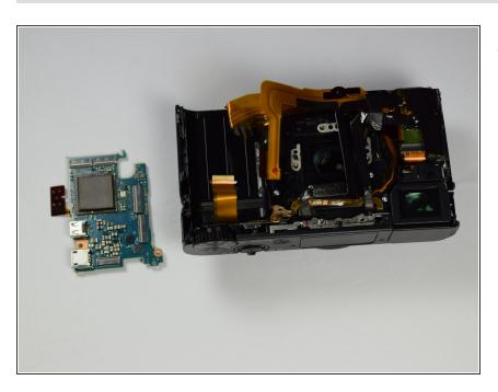
Viola! The motherboard is now removed and can be replaced with a new one.
