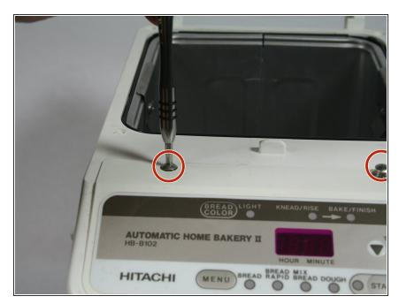
Begin by using a # 2 Phillips head screwdriver to remove the two 1.3 cm screws that secure the control panel onto the main body.
