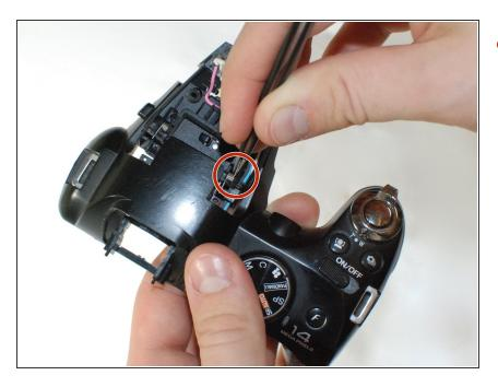
Use a pair of tweezers to remove the flash mechanism springs, then replace with the new springs.
