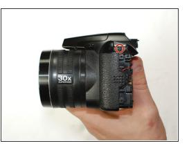
Remove the 3.5 mm Phillips #1 screws holding the top to allow access to the flash mechanism.
