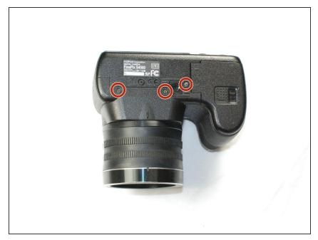
Remove the three 3.5 mm Phillips #1 screws in these locations on the bottom of the camera with a screwdriver.
