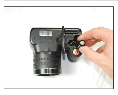
Remove batteries; make sure batteries are oriented correctly when replacing.
