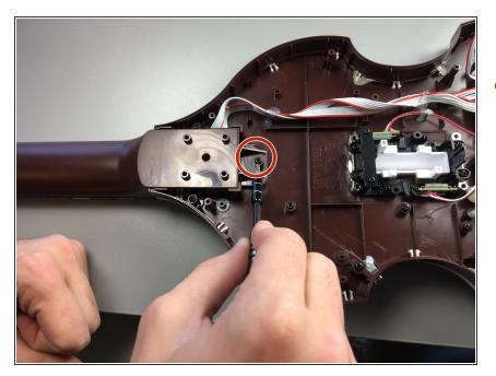
Using a J1 Phillips screwdriver, unscrew the 10mm screw at the base of the neck.
