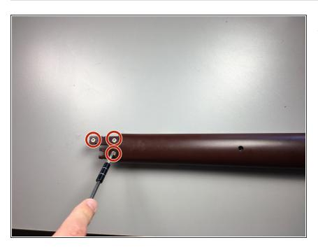
Use a J1 Phillips screwdriver to remove three silver 10mm screws at the top of the neck.
