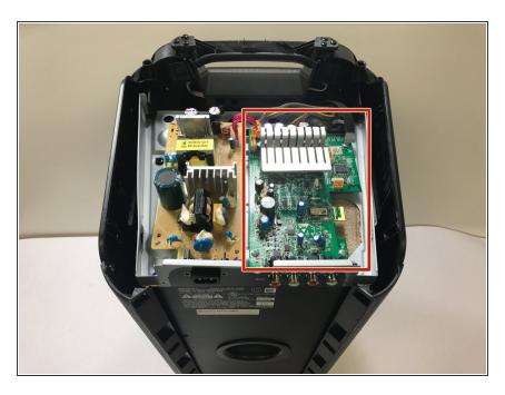
Find the large green motherboard, located underneath the top plastic housing of the speaker.
