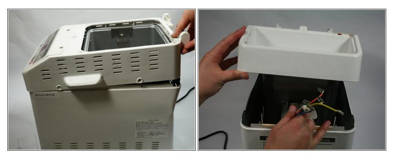
Now you can remove the top part of the assembly off by pulling straight up. Don't forget to gently pull your wires through.
