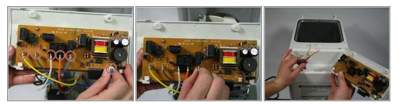
You will then have to disconnect the six wires that connect the motherboard to the device. This can be done by firmly grasping a connector and pulling straight out from the unit. Once all of the wires have been disconnected, set aside the control unit.
