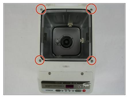
Unscrew the four 1.4 cm screws surrounding the slot for the bread pan.
