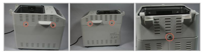
Remove the five 1cm screws that hold the the casing together. There will be two on each side, and one on the back.
