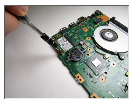
Remove the 5mm screw in the corner of the network card with a Phillips #0 screwdriver.
