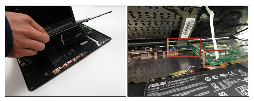
• Partially lift the panel up, revealing the two cables connected to the motherboard.
