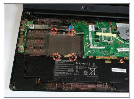
Remove the four 5mm screws from the hard drive mounting bracket using the Phillips #0 screwdriver.
