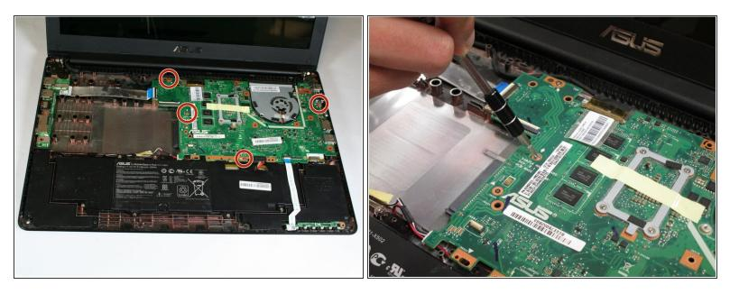
• Remove the four 5.5mm screws using the Phillips #0 screwdriver.
