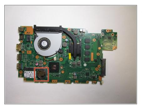
• Flip over the motherboard so that the CMOS battery is now visible.
