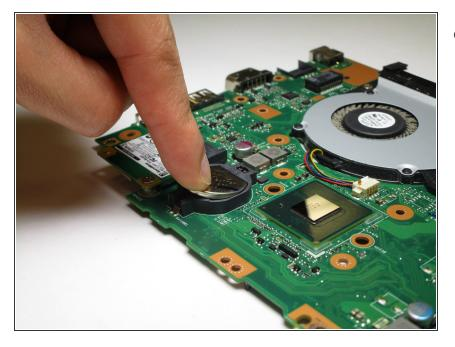
Insert the new CMOS battery (positive side up) into the slot using your finger.
