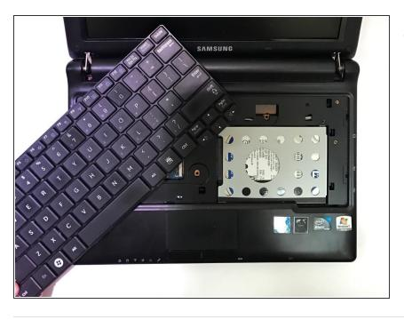
Manually remove the keyboard from the device.
