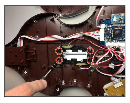
Use a J1 Phillips head screwdriver to remove the four 10mm screws at the corners of the black casing.
