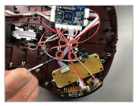
Use J1 Phillips screwdriver to remove the four 10mm screws on the whammy bars black cover.
