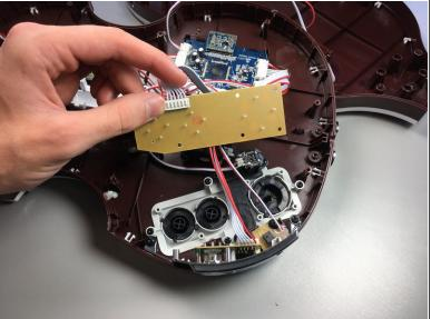
• Use a J1 Phillips screwdriver to remove the six screws 10mm around the brown button cover.
