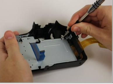
Unscrew the five 5mm screws on the panel that you just removed.
