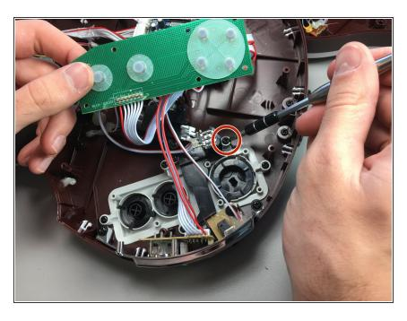
Use a J1 Phillips screwdriver to remove the 10mm screw on the toggle switch.
