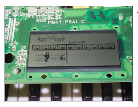
Flip over the component board to reveal the display that is currently connected to a green panel.
