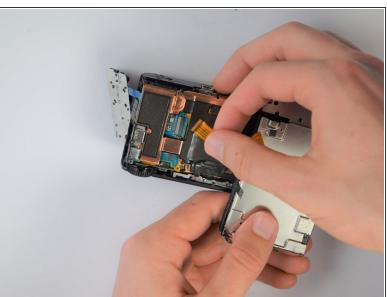
Carefully unplug ribbon connector to fully detach LCD screen assembly from camera
