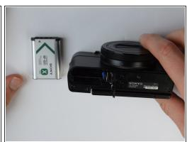
Remove battery by sliding the tab to open the cover
