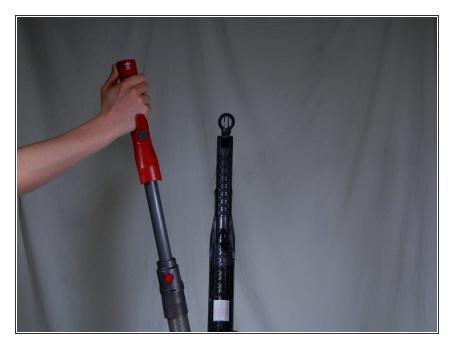
Gently pull up on red handle to separate the hose from the external hose of the Dyson.
