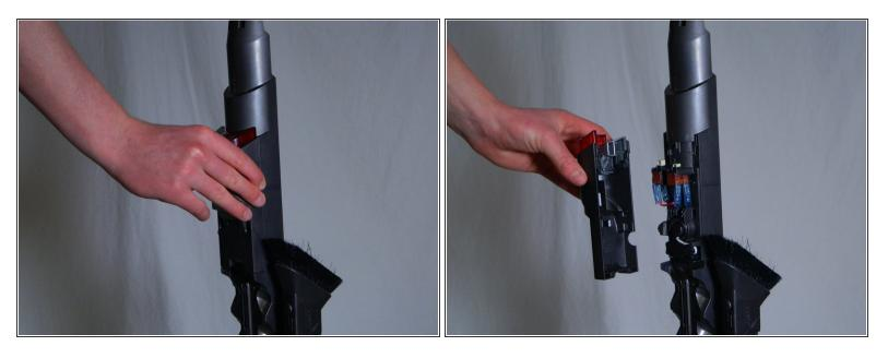
Pull on the plastic case below the power and brush bar buttons to separate it from the Dyson.
