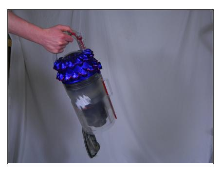
Press the red button again to open the bottom of the bin.
