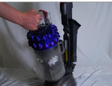
Push down the red button to remove the bin from the Dyson.
