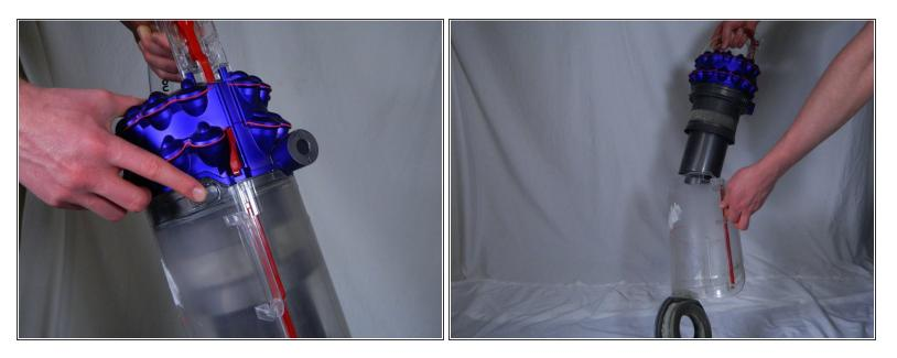
Press the grey button (where index finger is located) and slide the bin assembly out.
