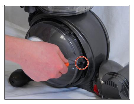
Continuing clockwise along the path, remove the next 18mm screw.
