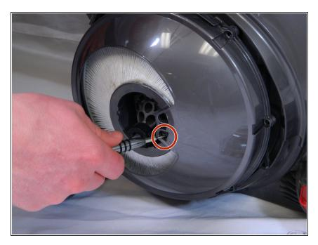
Then remove the final 18mm screw in the center. Once these have all been unscrewed, remove the filter with the cover. The filter and the cover should be attached to each other.
