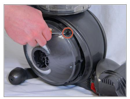
Next, remove the upper right 18mm screw along the perimeter of the circle.
