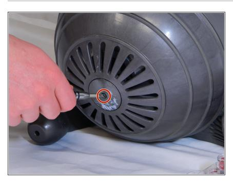
Remove the center 18mm screw from the Dyson Ball, then remove the covering.
