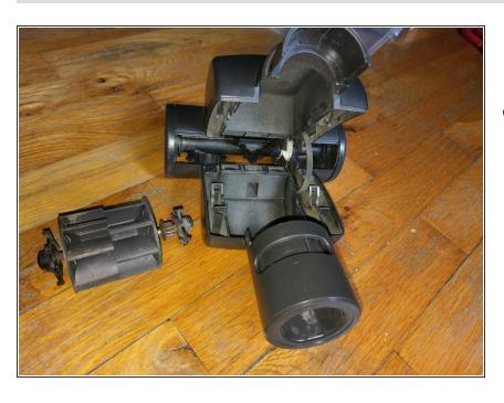
Now we remove the part that makes the unit spin. The fins are pulled by the vacuum suction and rotate the belt that moves the brush. To remove the Fin assembly, gently squeeze the little black plastic clips on either side. This does not take much force, do it gently as if you break the clips there is no way to repair them.
