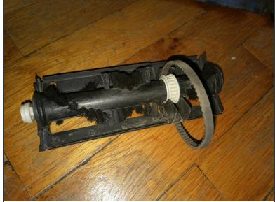
• To remove the brush axle from the brush assembly, pull the little white plastic end cap outward slightly (see second photo). Then you can just pull the brush axle out.
