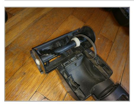
The top half of the unit that hinges upward can be removed by gently bending the plastic edges outward. You should be left with the bottom half and brush assembly as shown in the photo.
