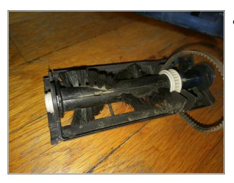
Just like the top half, the bottom half of the unit can be removed by gently bending the plastic fins on either side outward and sliding it off of the brush assembly. You will be left with what is shown in the photo.
