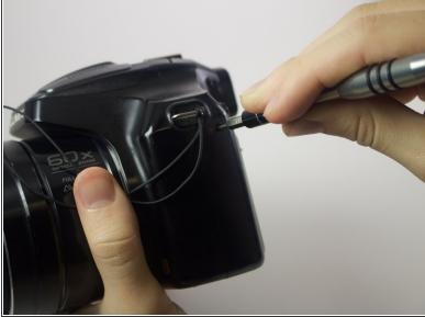
• Flip the camera over to the left side of the screen and unscrew the 5mm Phillips screw found there.
