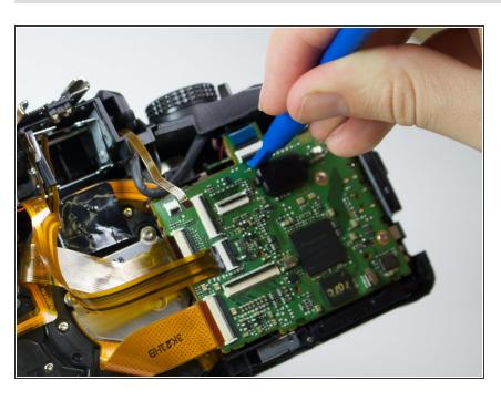
Using a plastic opening tool, flip up the switch on the ZIF connector underneath the operations unit and
