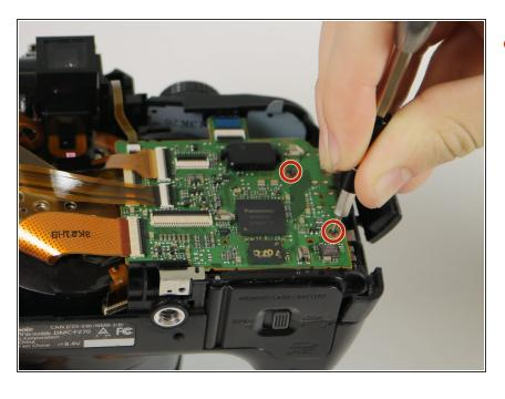
Using a Torx driver, unscrew the two 5mm Phillipd screws on the motherboard
