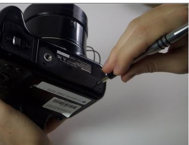
Turn the camera upside down and unscrew the three 5mm screws found on the bottom.
