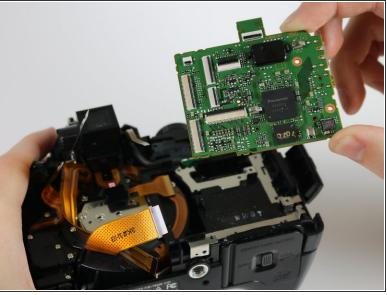
Once the screws and the ribbon cables have been removed, lift the mother board from its slot.
