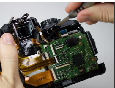
Unscrew one 10mm Phillips screw to the right and underneath the viewfinder.
