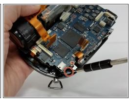
• Remove the three black screws (5 mm, Phillips #00) connecting the frame to the disc housing.
